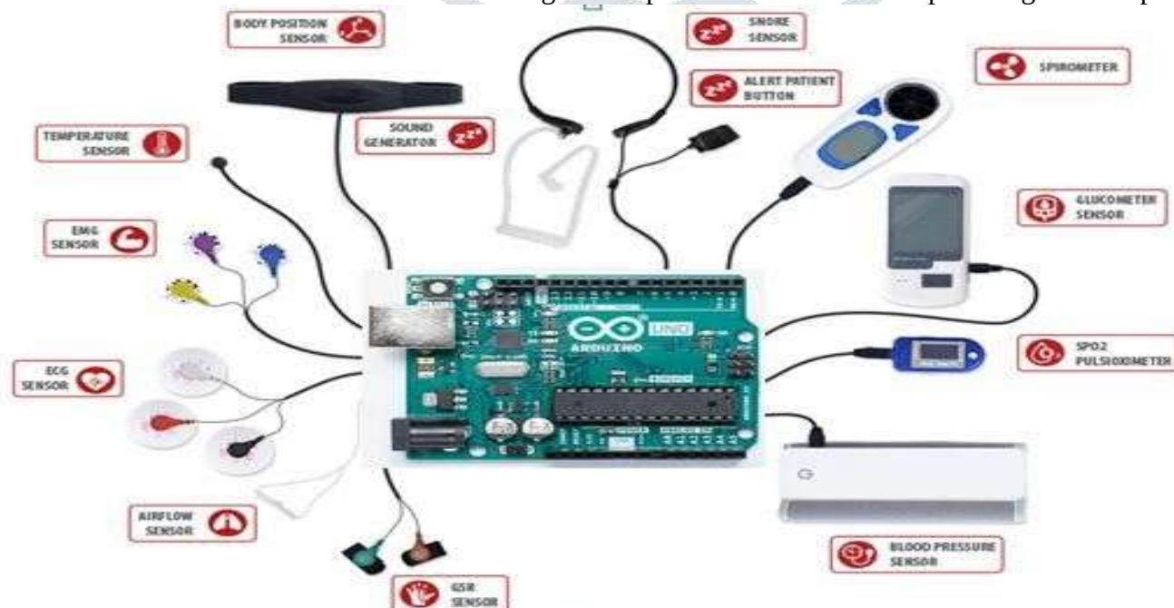
Figure 7: IOT Based Patient Remote Monitoring System
