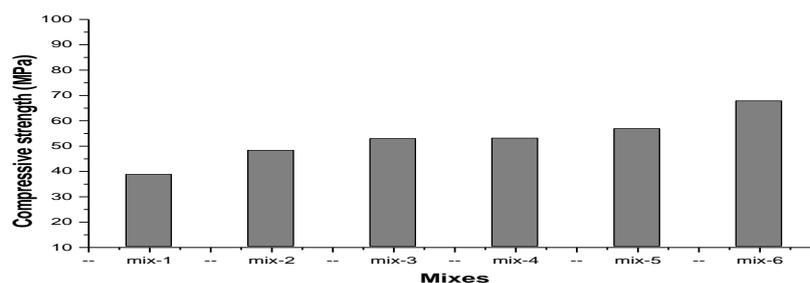
From the above graph, mix prepared with the combination of LWF.A and NWC.A with addition of 2% steel fibers and 10 % silica fume showed the highest compressive strength of 68Mpa. And mix with All lightweight aggregates without addition of any admixture or fibre shows the lowest value of 39Mpa.
