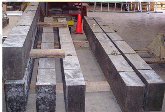
Fig. 2. Geopolymer concrete beams by Sumajouw et al. [15].
