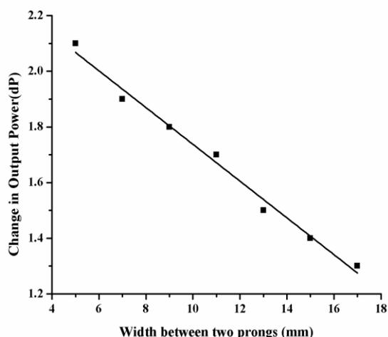
**Fig.-3:** Relation between Width between two prongs Vs Change in output power (dP)
