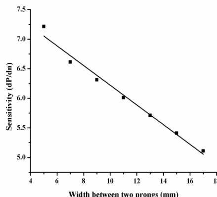
**Fig.-6:** Relation between Width between two prongs Vs Sensitivity (dP/dn)
