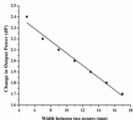
**Fig.-5:** Relation between Width between two prongs Vs Change in output power (dP)
