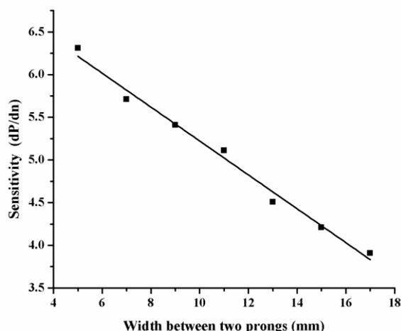
**Fig.-4:** Relation between Width between two prongs Vs Sensitivity (dP/dn)
