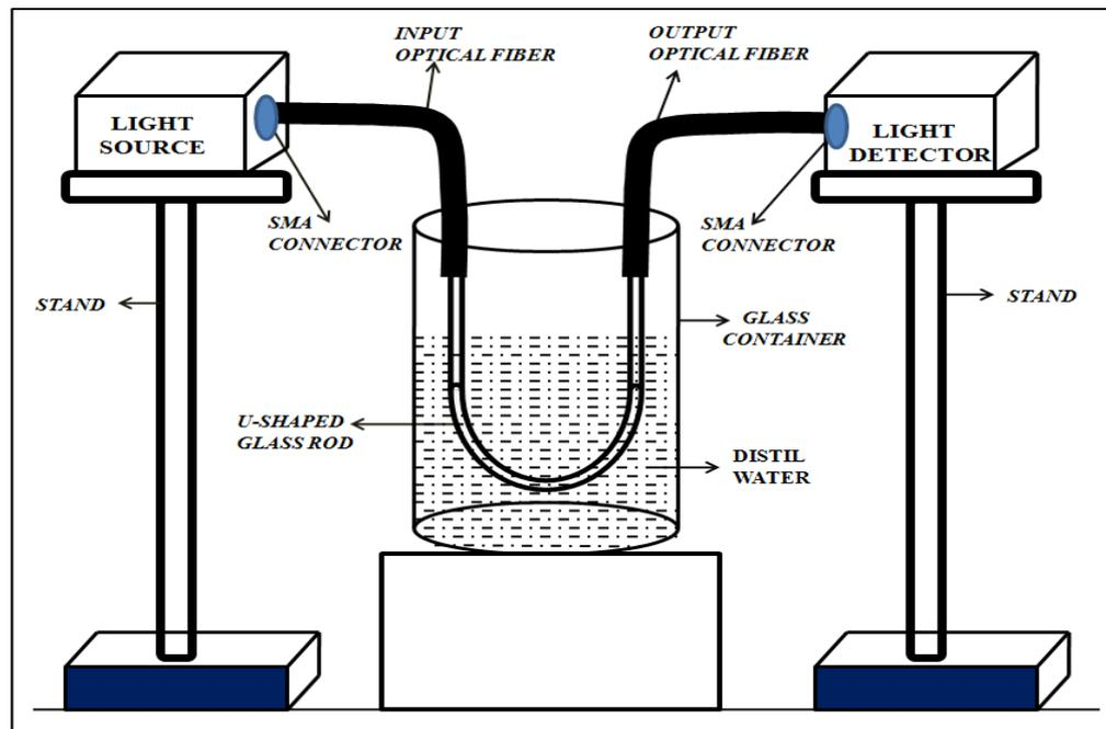
Fig.1: Experimental arrangement of U-shaped glass rod based Fiber Optic Refractometer
