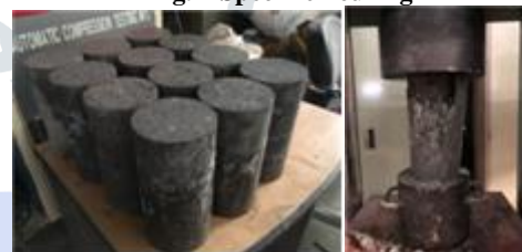
Fig. 3 Experiments of compressive strength of specimens
