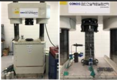
Fig. 7 Column compression test
