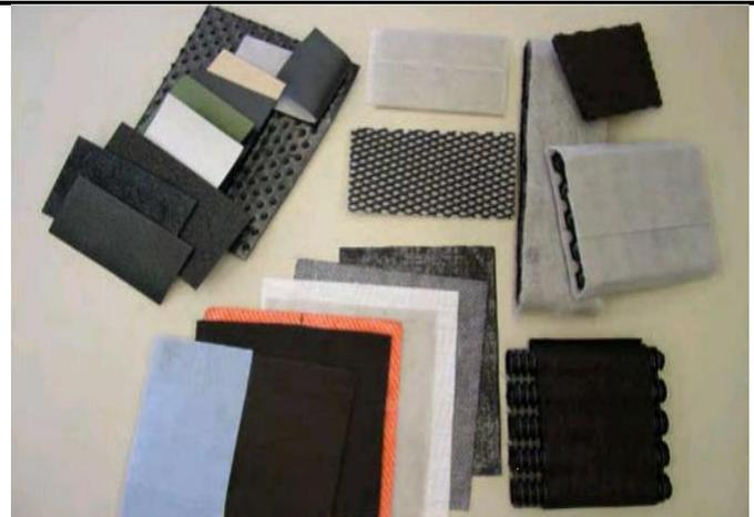
Fig. 2 – Types of Geosynthetic
