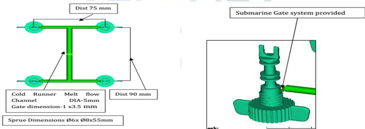
**Fig No 6 Runner Model and Layout (3<sup>rd</sup> Iteration)**
