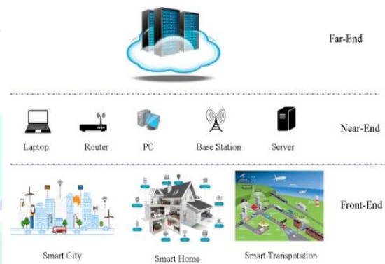
Fig 5: A typical architecture of edge computing networks
