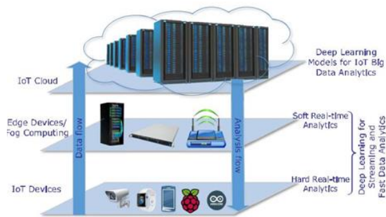
Figure1: IoT data generation at different levels and deep learning models to address their knowledge abstraction
