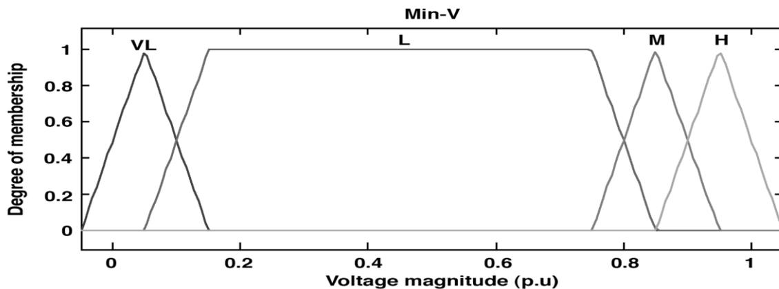
Fig. 7 Absolute minimum voltage input membership function
