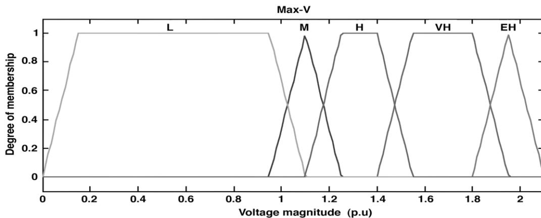
Fig. 3 Maximum voltage input membership function
