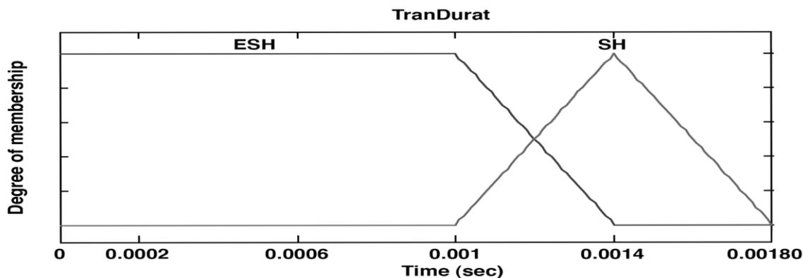
Fig. 6 Transient duration input membership functions
