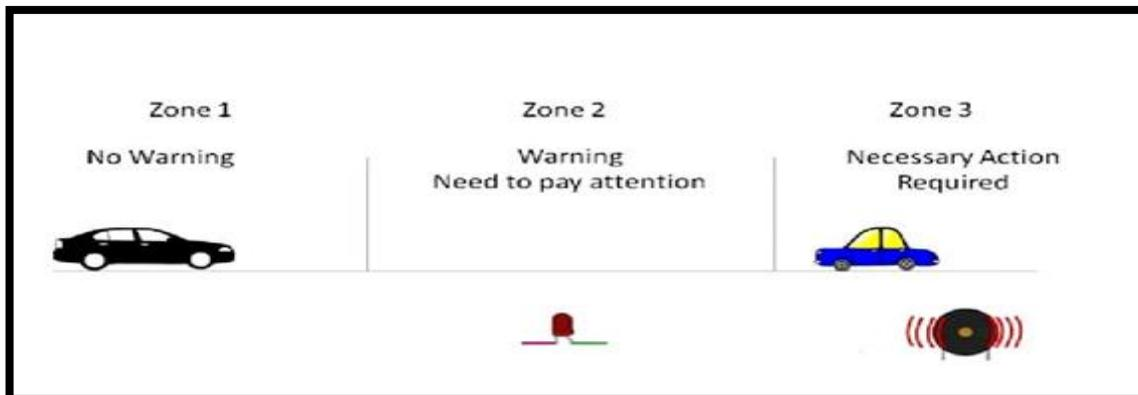
Figure1.Collision Detection Warning System
