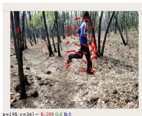
Figure 5 Output of Detected Motion using Motion detection algorithm
