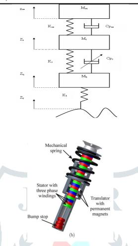
Fig: schematic view of a semi active suspension system
