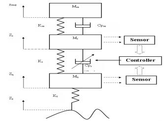
Fig. Quarter Car of Active Suspension system.
