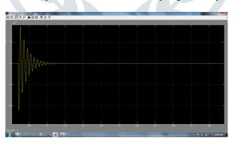
graph no.3. velocity of unsprung mass using active system.
