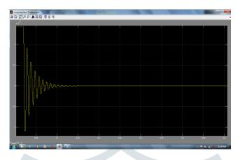
As shown on the graph the displacement of unsprung mass in case of active suspension system is upto the  $1.45*10^{-5}$ . As this maximum displacement of unsprung mass is less than the maximum displacement of unsprung mass in case of passive system as shown in the graph no.1
