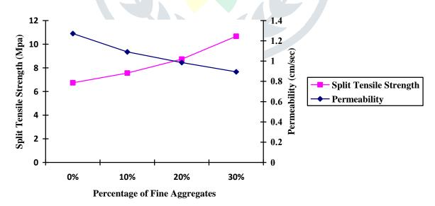
From the above graphs it has been observed that the increase in the volume of fine aggregates results in decrease in permeability and increase in the strength (Compressive strength, Split tensile strength). The optimum mix is obtained for the percentage of fine aggregates ranging between 20-25 % for optimum permeability as well as optimum compressive strength.
