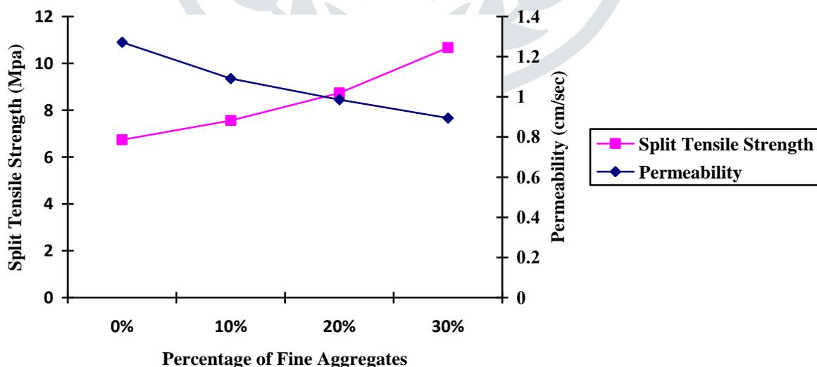
From the above graphs it has been observed that the increase in the volume of fine aggregates results in decrease in permeability and increase in the strength (Compressive strength, Split tensile strength). The optimum mix is obtained for the percentage of fine aggregates ranging between 20-25 % for optimum permeability as well as optimum compressive strength.
