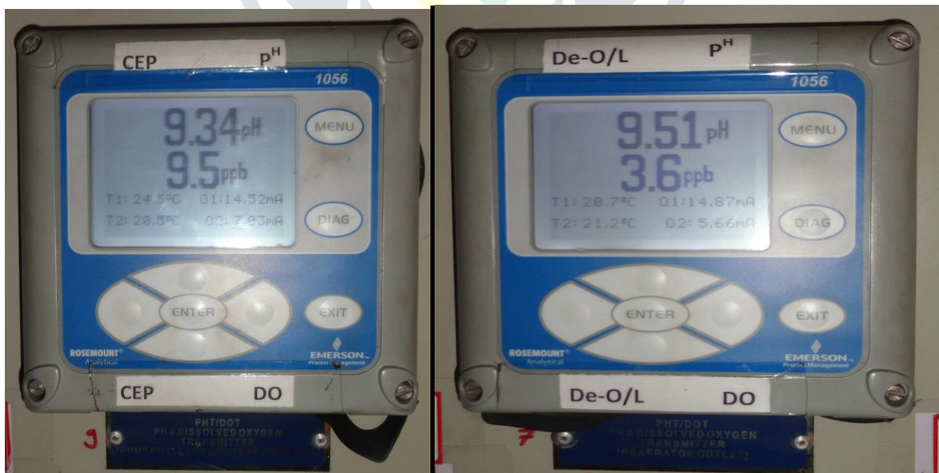
Figure 8 CEP DO and Deaerator DO measured in online reading in SWAS lab
