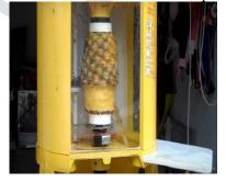
B. Pineapple cutting machine: - This is a machine which cuts pineapple into round pieces or we can say slice. For this pineapple must be peeled or without peeled. After peeling the pineapple is placed in this machine and makes the slice.
