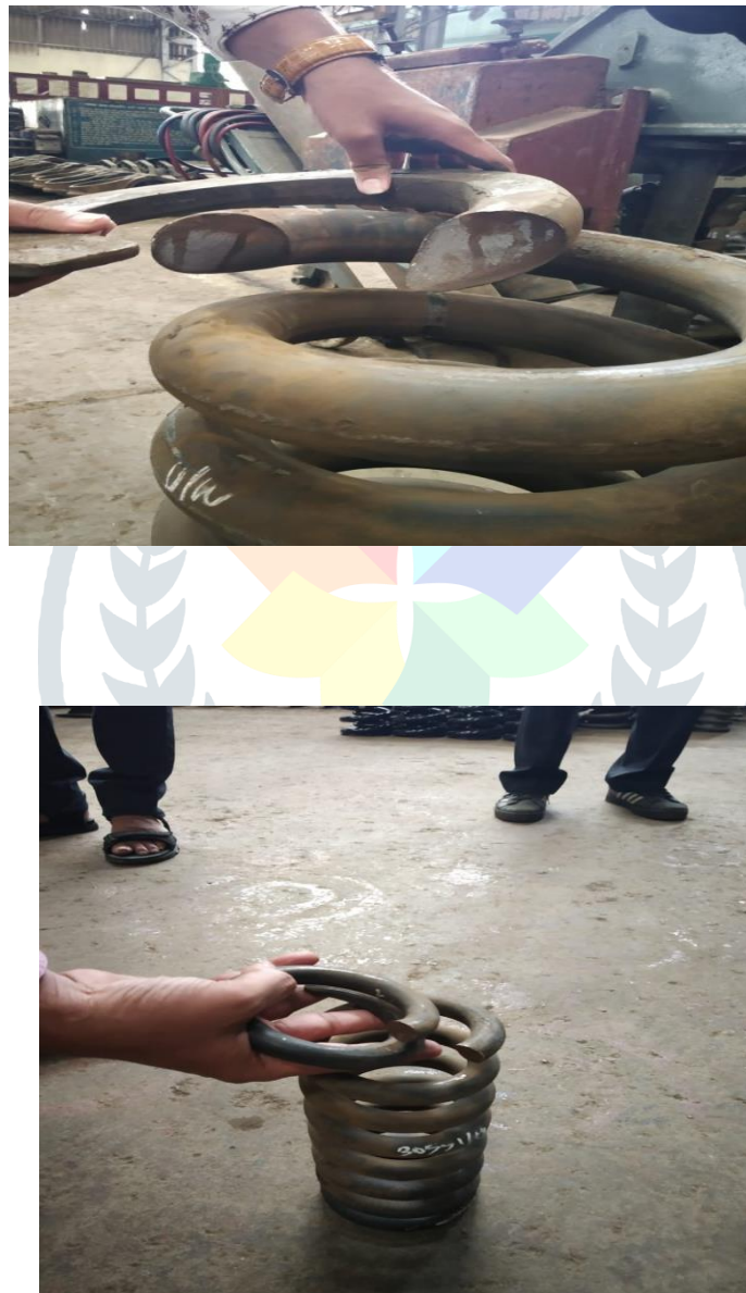
Fig.Broken Primary Spring
