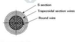
(c) Locked-coil cable
