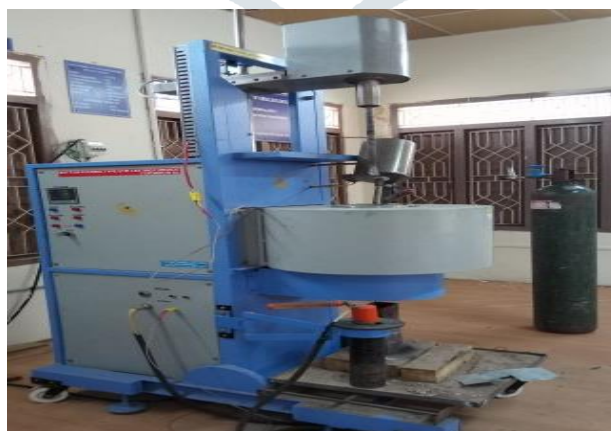
Fig.5. Bottom type Stir casting equipment
