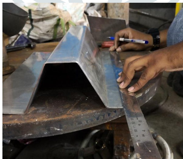
Fig. 25. Removing excess material from the sheet after bending
