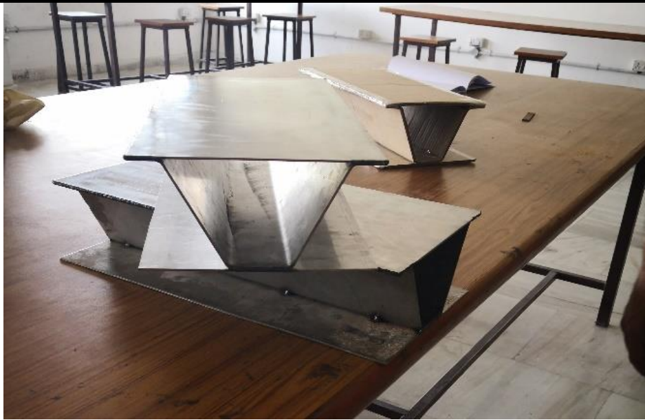
Fig. 23. Finished product of corrugated sandwich panel.
