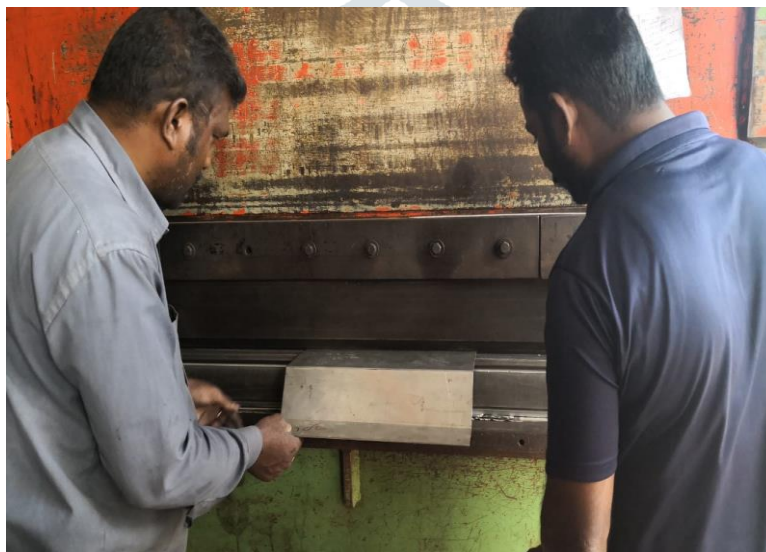
Fig. 24. Bending the sheet at 60° angle
