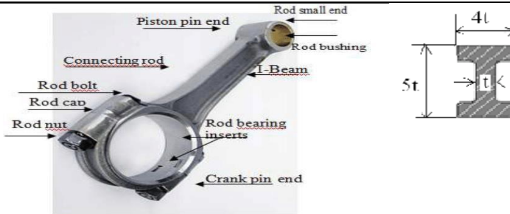
Fig1: Connecting rod and its cross section
