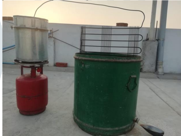
Fig : Pyrolysis Reactor Setup
