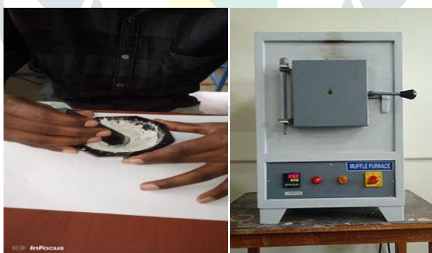
Fig 1: Reducing the size of nanoparticles by using agate motor
