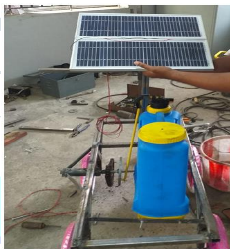
Fig 6: Arrangement of Solar panel
