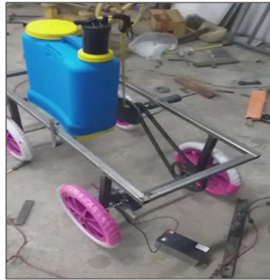
Fig 4: Installing the tank
