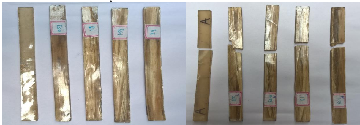
Fig 6.1 Specimens Subjected to Tensile Testing (Before and after testing)
