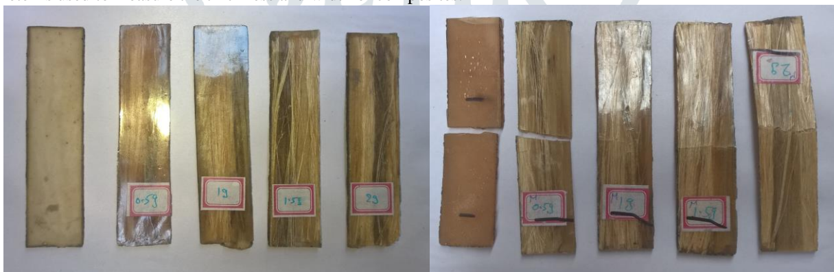
Fig 6.2: Specimens Subjected to Flexural Testing (Before and after testing)
