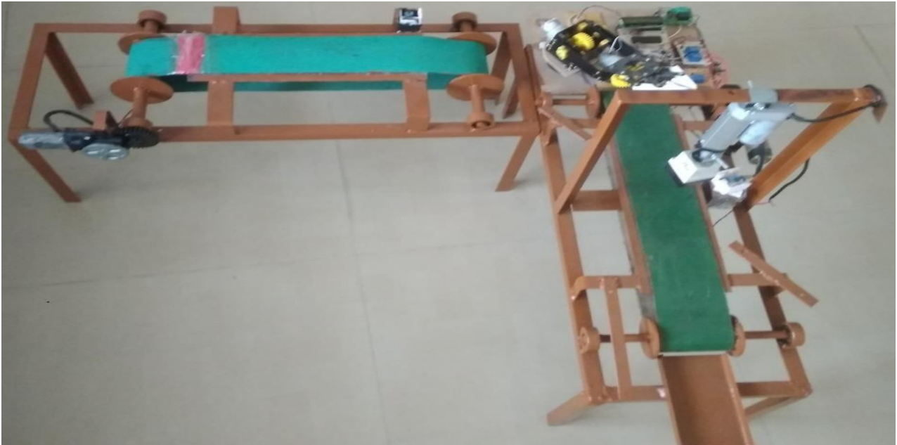
Fig 3.7: Design and fabrication of L-shaped automated pick-and-place robot arm with punching operation
