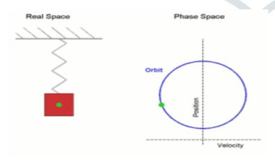
A simple harmonic oscillator, consisting of a weight attached to one end of a spring, is shown. The other end of the spring is connected to a rigid support such as a wall. If the system is left at rest at the equilibrium position then there is no net force acting on the mass. However, if the mass is displaced from the equilibrium position, the spring exerts a restoring elastic force that obeys Hooke's law.
