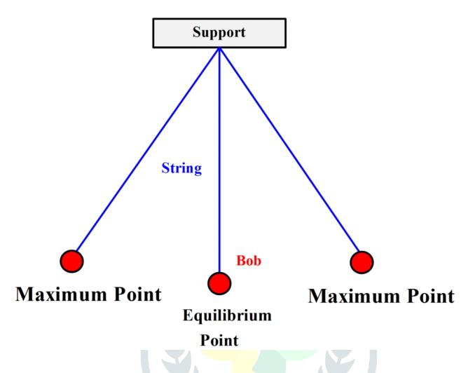
One type of simple harmonic oscillator is a simple pendulum. A simple pendulum is an object that has a small mass, which is suspended by a light wire or string.
