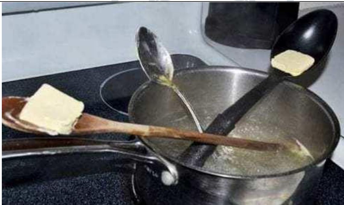
Fig 2. STAGE TWO SHOWING RATE OF ONE DIMENSIONAL CONDUCTION OF HEAT
