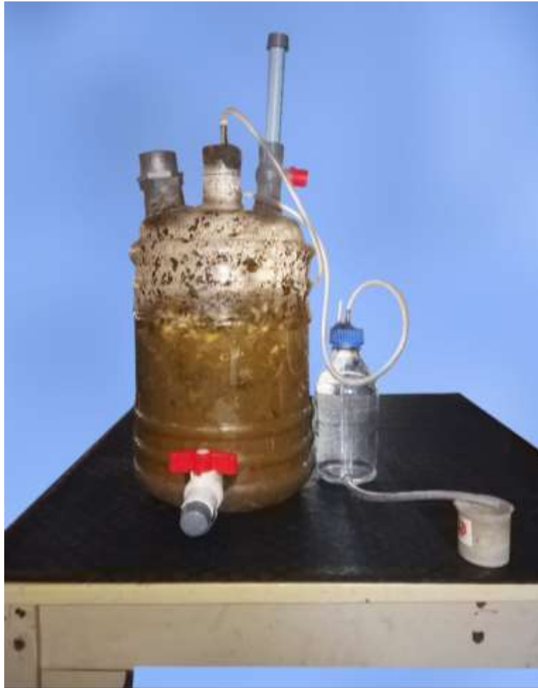
Figure 1 Batch Reactor with Gas Collection System
