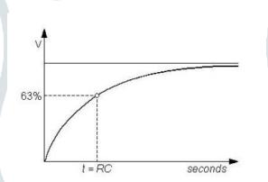
Larger capacitors take longer to charge, and therefore will create larger time constants. The capacitance in an RC circuit is related to the time constant by the equation:  $TC = R \times C$
