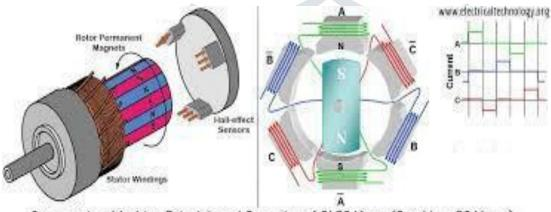
Construction, Working Principle and Operation of BLDE Motor (Brushless DE Motor)
