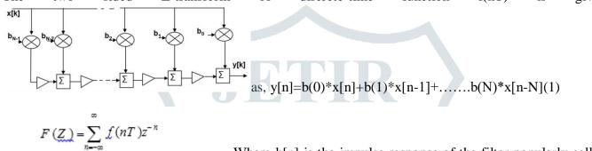
Where h[n] is the impulse response of the filter popularly called the filter coefficients in case of FIR filters. It can be seen from the basic filtering architecture that the basic operation consists of multiplication and addition which are the two major mathematical operations and are well performed by the Multiply & Accumulate units (MAC)
