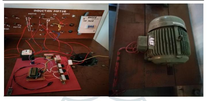
This system consists of various sensors and measurement circuits which measure the parameters of the motor continuously. These sensors have to be compatible with the Microcontroller i.e., their output voltage range should be between 0-5V DC. So, some of the sensors needs signal conditioning equipment as we are measuring the AC
