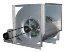
The blower may operate at a single speed, offer a variety of set speeds, or be driven by a variable-frequency drive to allow a wide range of air flow rates. Flow rate may also be controlled by inlet vanes or outlet dampers on the fan. Some residential air handlers in USA (central "furnaces" or "air conditioners") use a brushless DC electric motor that has variable speed capabilities.
