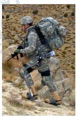
The purpose of exoskeleton is to provide forces against to external load carried by user during walking, sitting, and standing motions. Thus, it supports walking and large portion of load carrying by the human. Also it makes the user to spend less energy.
