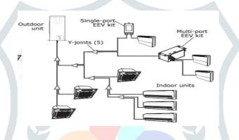
Normally copper pipe is use. This is different in diameter. Normally 10 fit in length is available for piping Basic length of pipe in diameter(mm) is 6,10,12,16,19,22,28,35,42 Refrigerant piping diameter, thickness, and temper is selected according to length.
