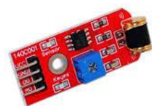
Figure 4. Heartbeat sensing element
