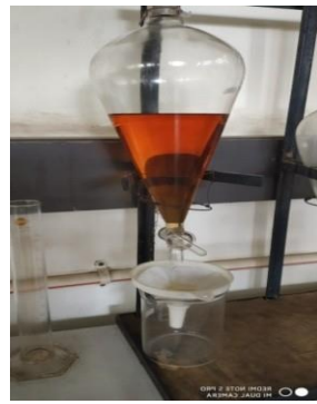
Fig 5. Bio diesel filtration
