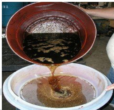
Figure 1. Filtration of Raw waste cooking oil
