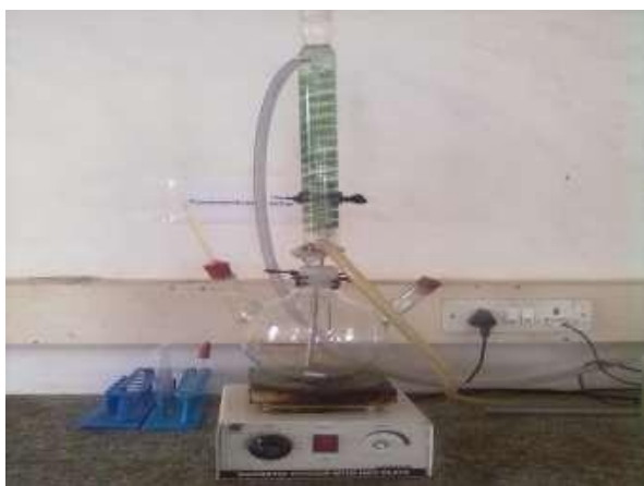
4.1 Experimental Trans-esterification setup Fig. 4.2 : Separation of free fatty acid
