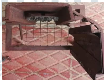
Fig 2 - Feeding Cup When Second Half of the Cup Is Open
