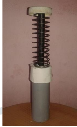
Fig 7: Model of the Power Generating Suspension System
