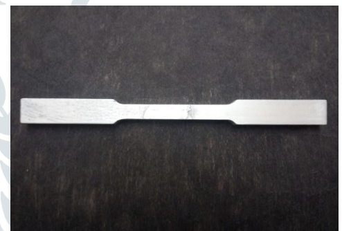
Figure 3.5: Tensile Test Specimen.
