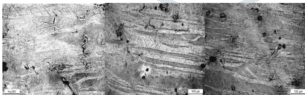
Fig.4: Microstructure of copper alloy after cryorolling
