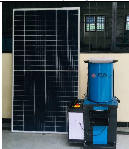
Figure no: 8.3 Developed model of the shredder machine
