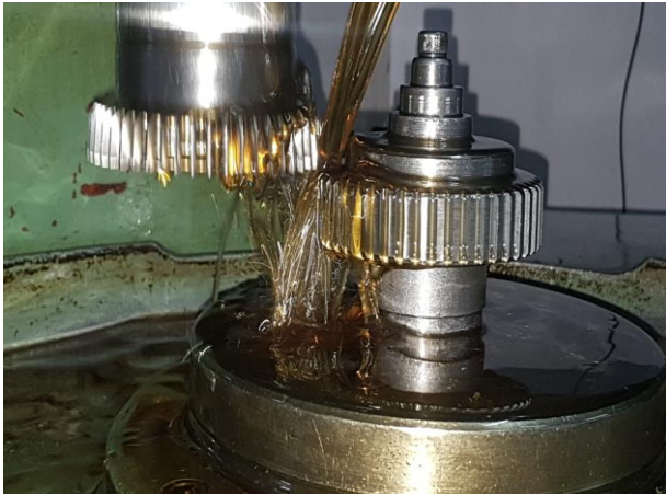
Fig 2: Vertical milling of spur gear
