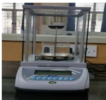
Fig6: Density testing apparatus
