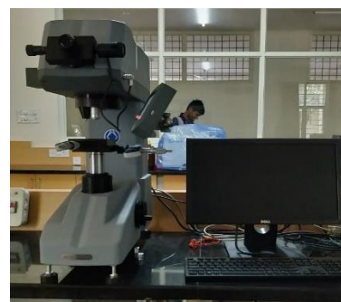
Fig 7: Computerized Micro Hardness Testing Machine
