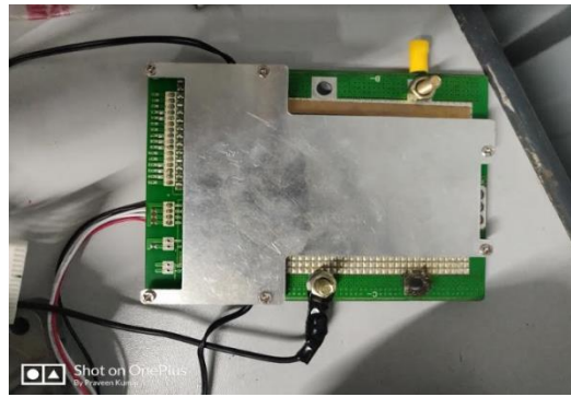
Figure 4- Battery Management System
