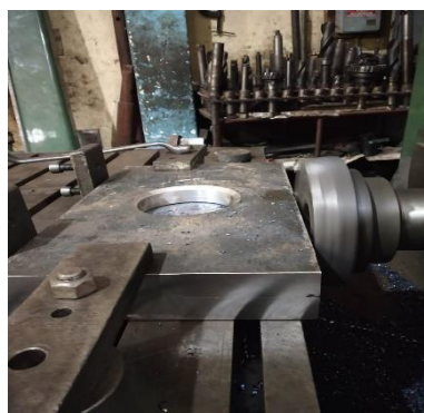
Fig.2 Machining of Top and Bottom Plates
