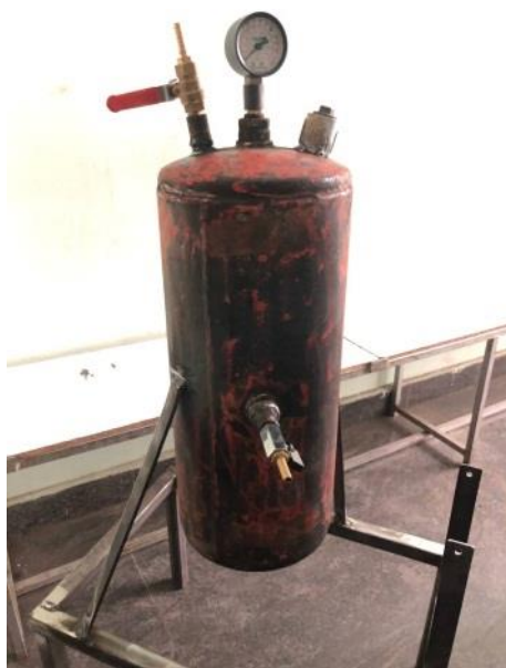
Fig. 1 Boiler drum equipped with mountings
