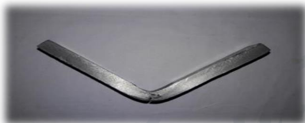
Fig. 3.14 Flexural Sample-1 Specimen after Testing
