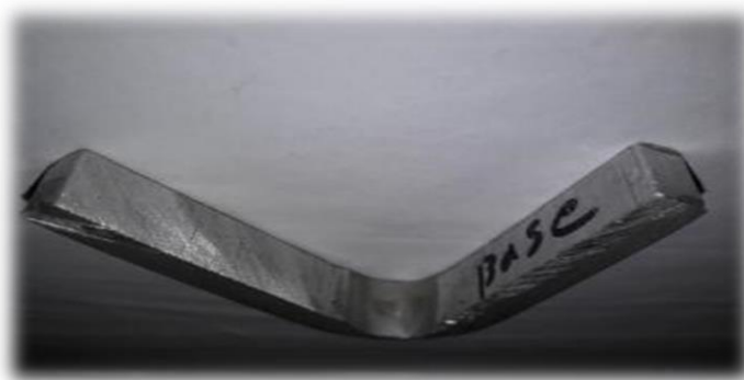
Fig. 3.13 Flexural Base Metal Specimen after Testing
