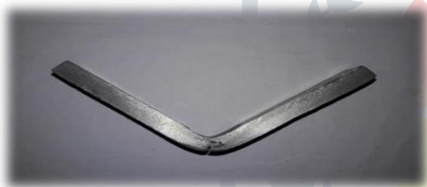
Fig. 3.16 Flexural Sample-3 Specimen after Testing
