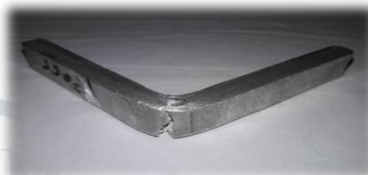
Fig. 3.15 Flexural Sample-2 Specimen after Testing
