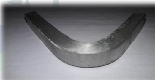
Fig. 3.17 Flexural Sample-4 Specimen after Testing
